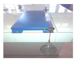
Figure.1: Modified instrument used for the measurement of tensile strength.
